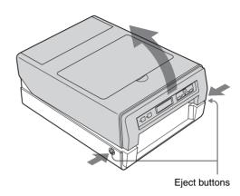
**5** If the head cleaning unit is open, push the head cleaning unit without touching the print head to close it.
